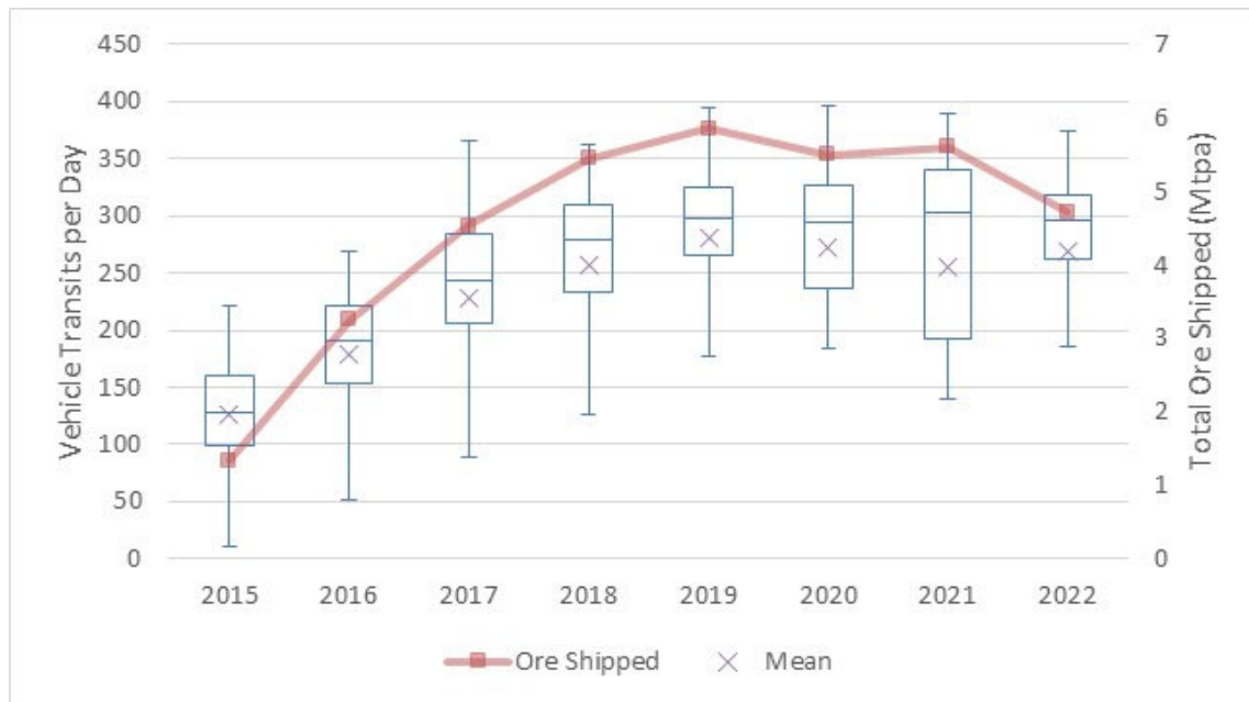
Figure 4.7: Trends in Vehicle Transits on the Tote Road and Total Ore Shipped from 2015 to 2022
