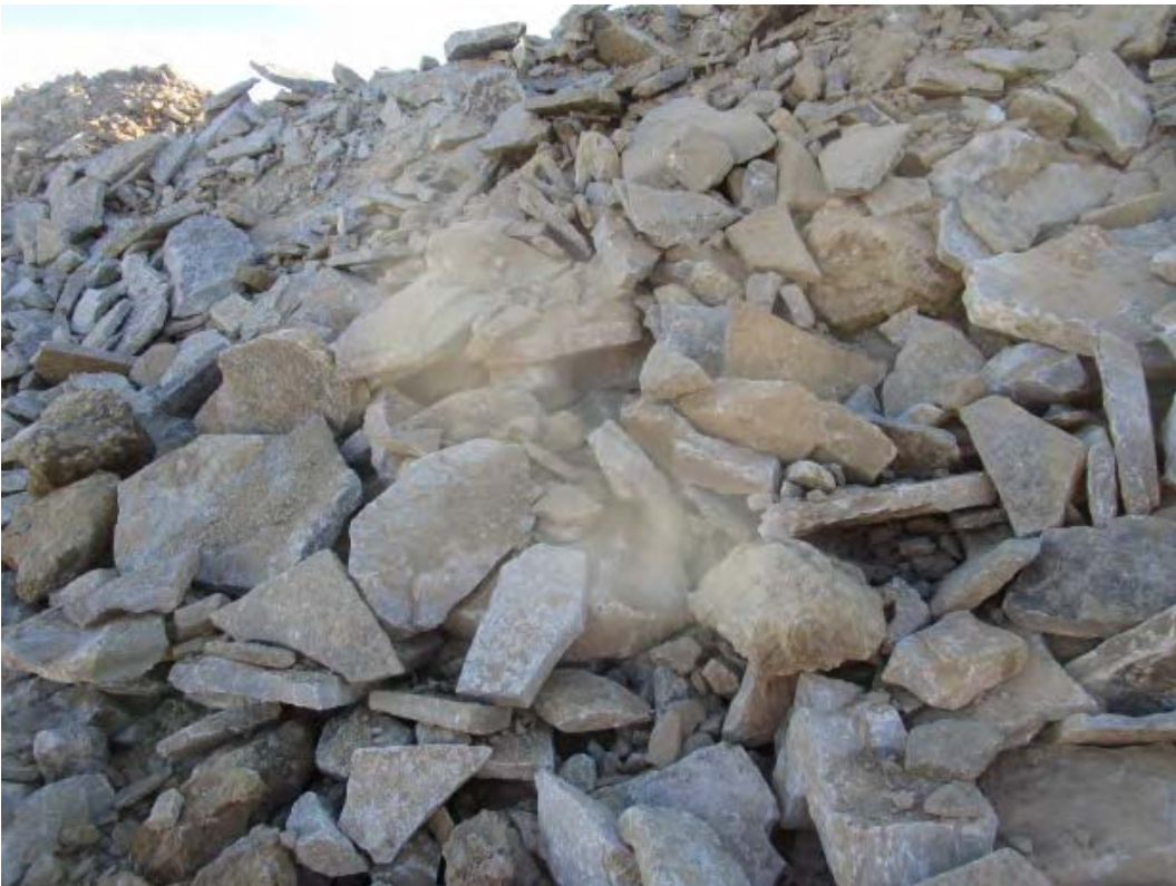
35. Typical Rock Used as Fill from km 76
