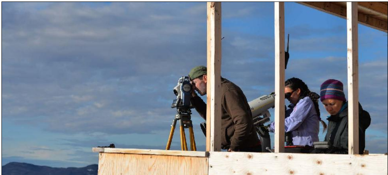
FIGURE 10. The theodolite was used to take location fixes on narwhals, other marine mammals, and vessels in the study area.
