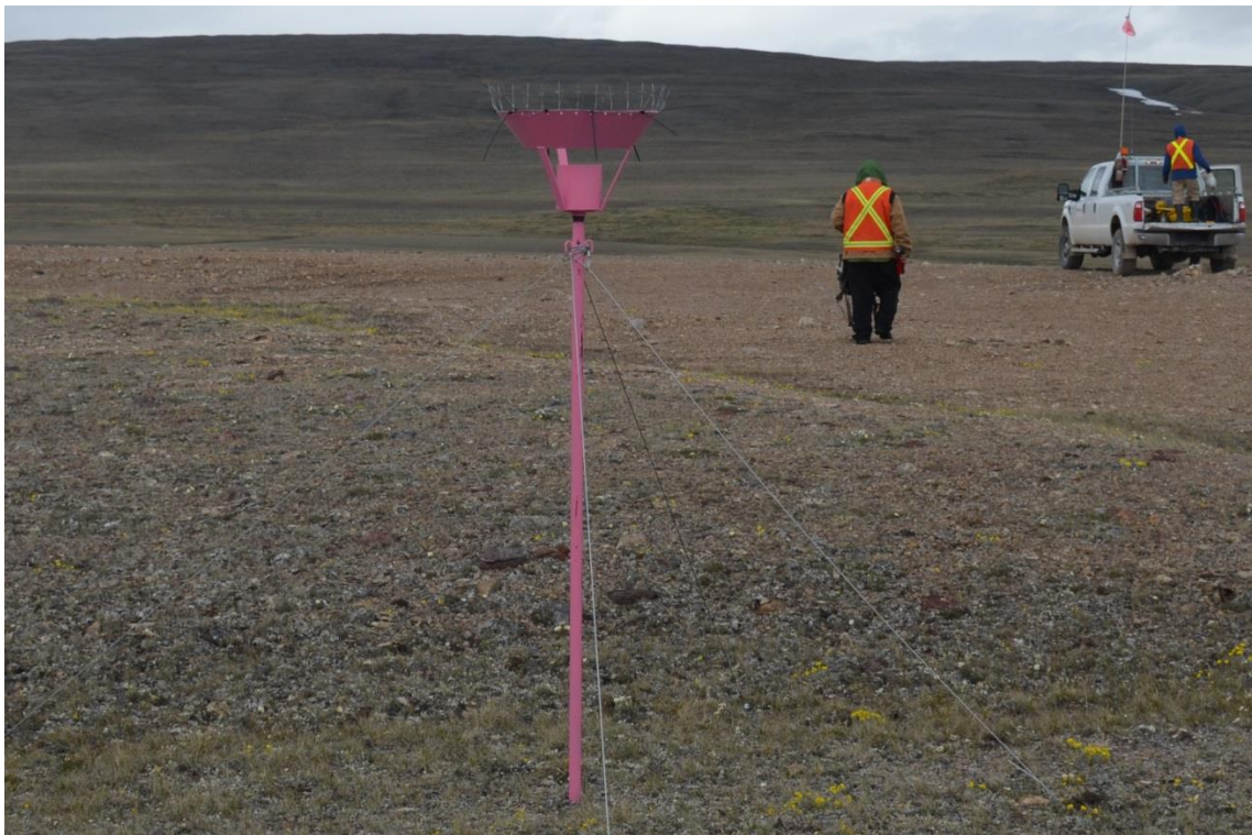
Photo 1. Dust fall collector sampling apparatus, July 10, 2013.
