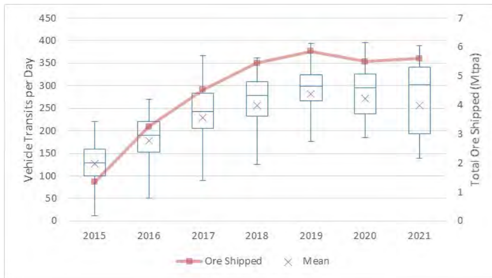
Figure 6-1. Mean ore haul and non-haul vehicle transits per day and total ore shipped between 2015 and 2021.
