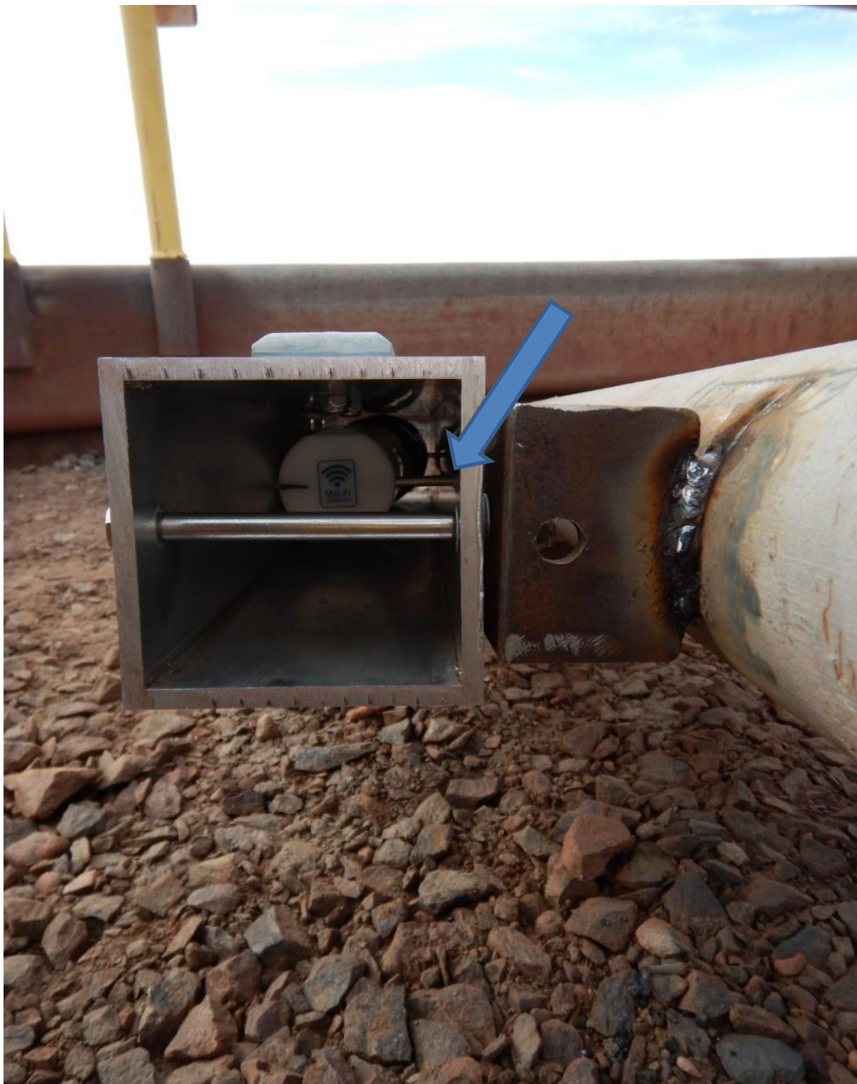
Figure 4: Hardware attaching aluminum tube to L brackets and view of the primary tide gauge mounted in the tube. Arrow shows location of the 1/4" bolt that should pass through the end cap of the primary tide gauge. Note that the redundant tide gauge is not shown in this photo, but would be sitting to the right of the primary tide gauge in this photo.
