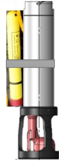
Figure 3: Configuration of an RBRsolo hose clamped to an RBRconcerto.
