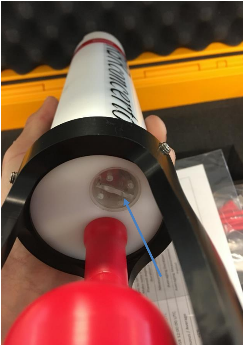
Figure 7: Pressure sensor location, shown by the arrow, on the downward facing end of the primary tide gauge
