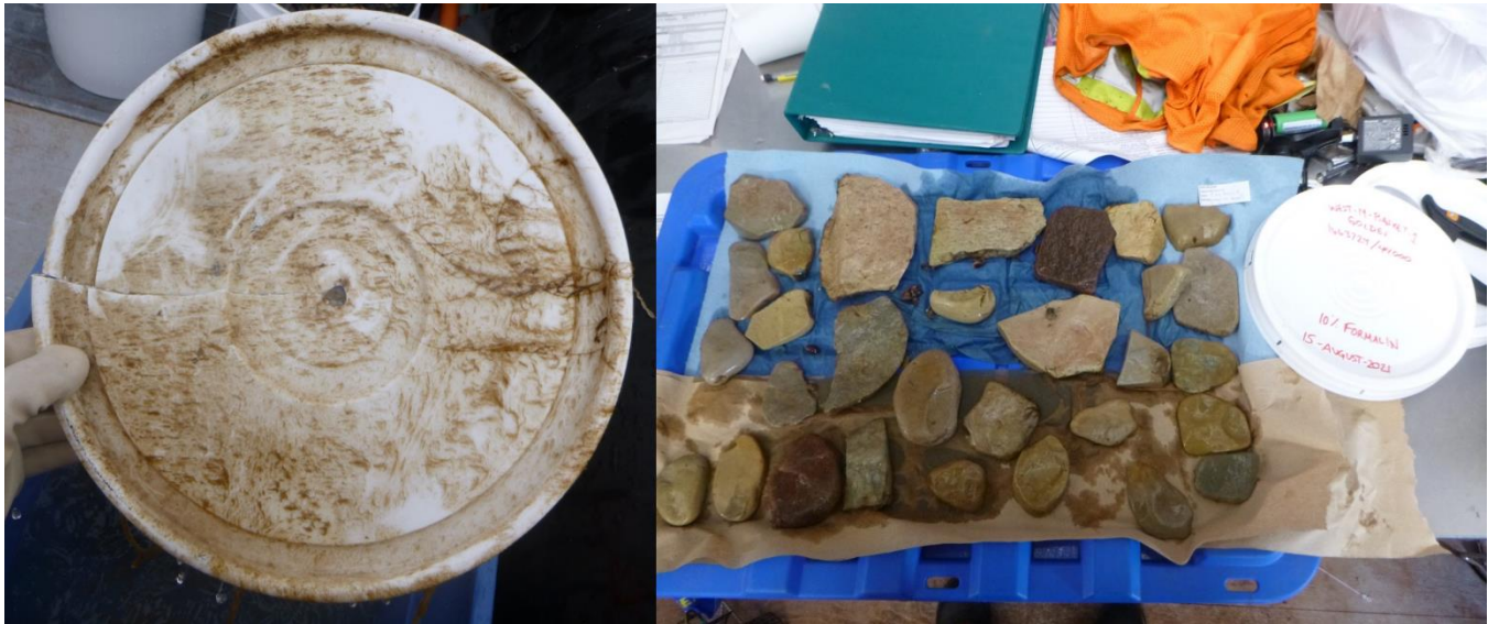
Figure 8-6: a) Settlement Plate Collected from the Centre-D Station on the Freight Dock and b) Rocks from Settlement Basket collected from the West-M Station on the Freight Dock, following One Year Deployment (14 and 15 August 2021)
