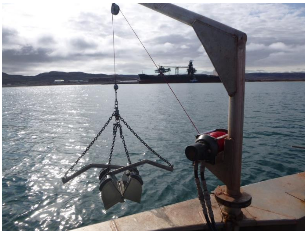
Photo 2 – Van Veen grab set and ready for deployment on 10 August 2021.
