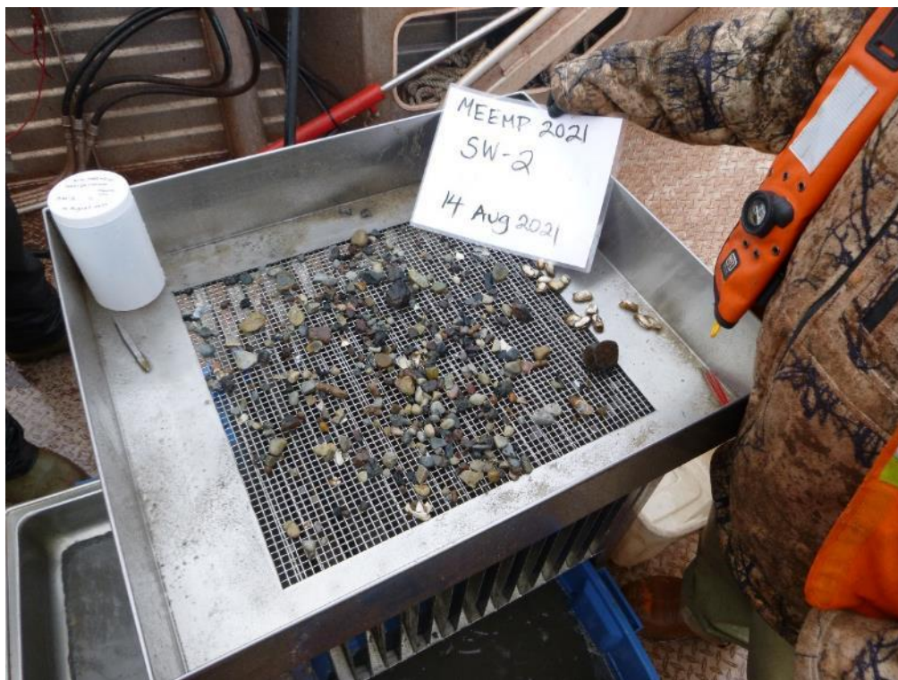
Photo 3 – Benthic sample on 1.0 cm sieve, collected at station SW-2 on 14 August 2021.
