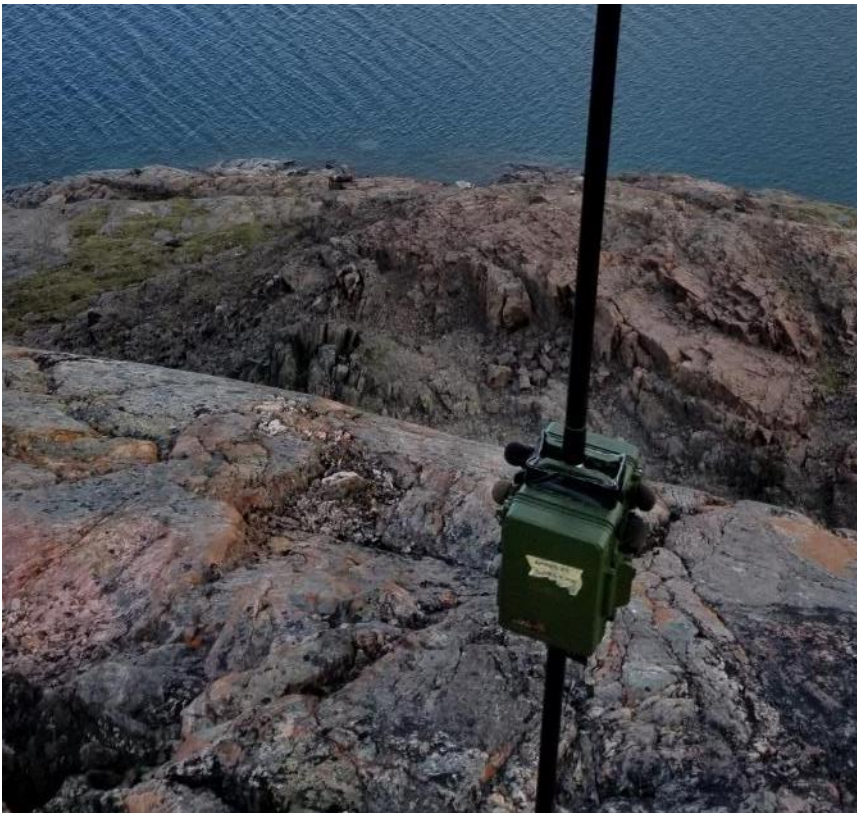
Photograph 5.2: Two SM4 acoustic recorders mounted back-to-back on a fiberglass pole. The shoreline location of the Inuit hunting camp is visible in the background.
