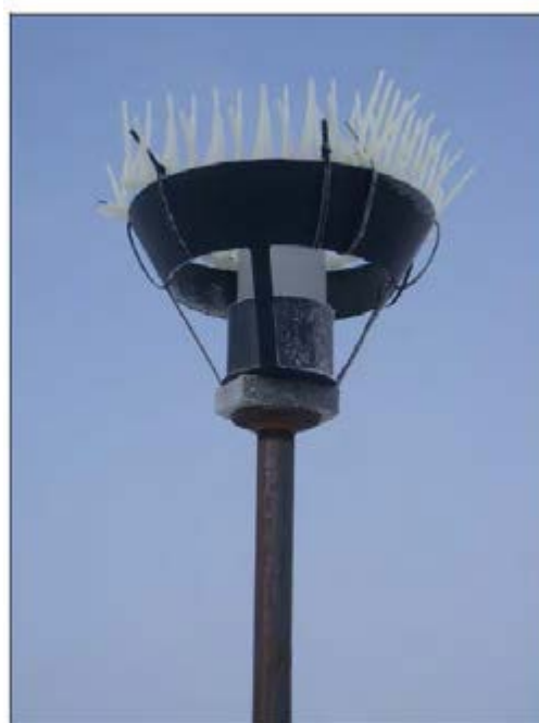
Photo 1: Dustfall collector sampling apparatus (from Rescan 2012).
