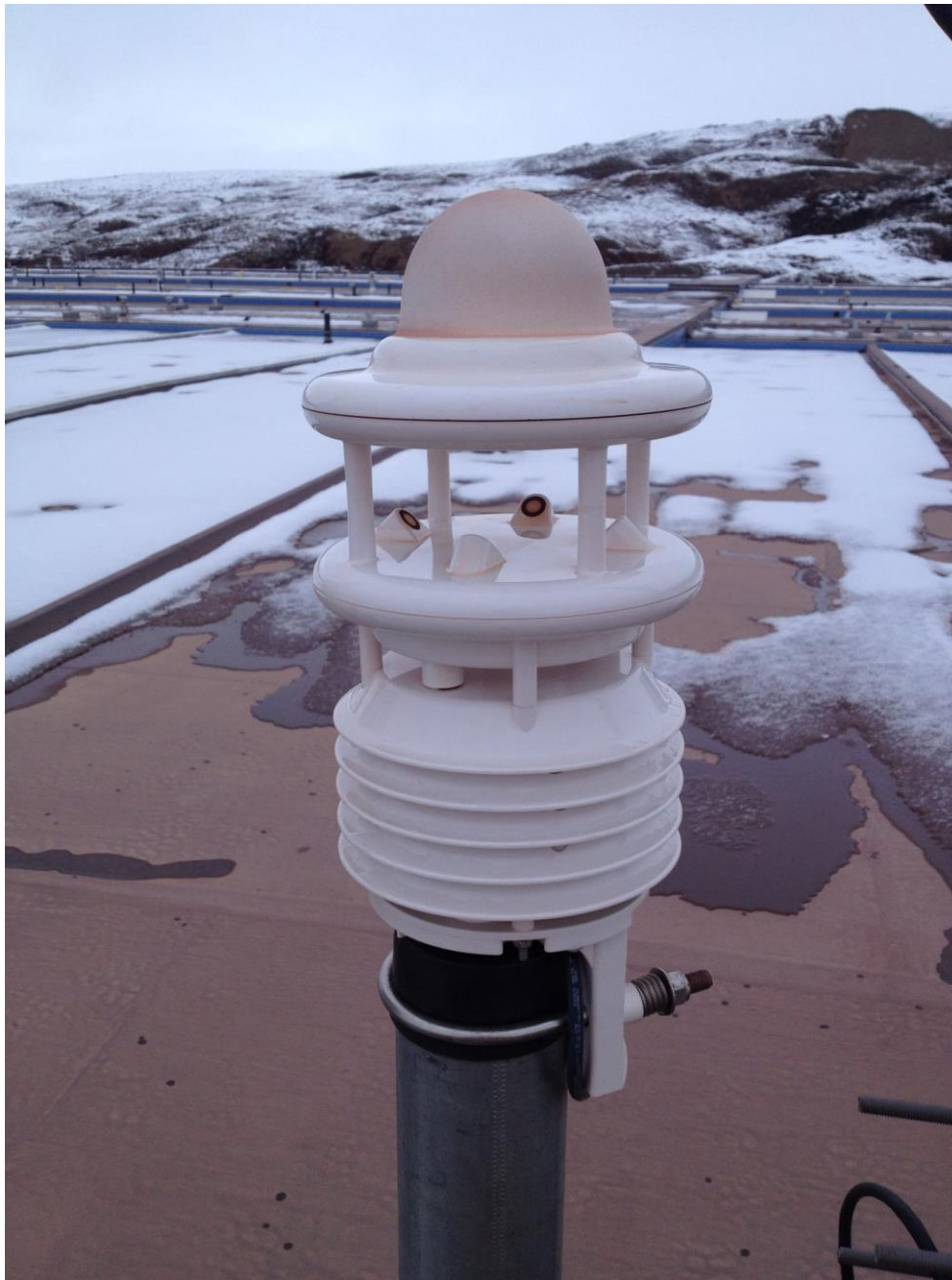
Figure 16: Current condition of WS600-UMB Lufft sensor at Mary River Camp
