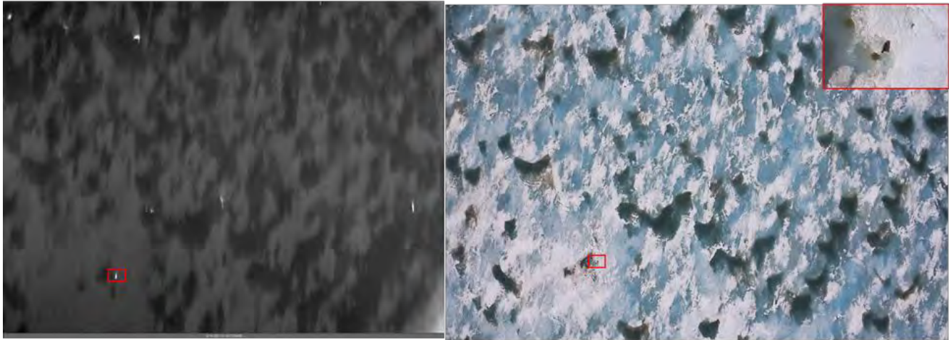
Figure 15: Example of paired aerial images obtained from infrared camera (left) and digital single-lens reflex camera (right) during the 2021 RSASP on 14 June demonstrating the efficiency of infrared imagery with visual photographs in poor sighting conditions.
