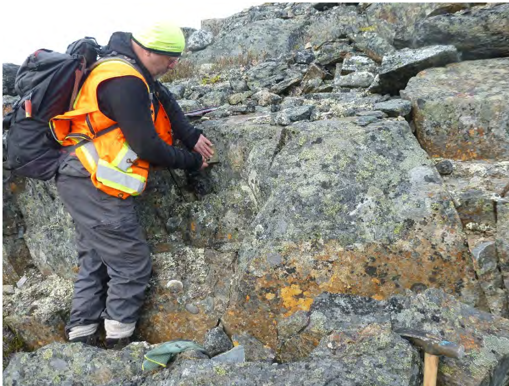
PHOTO 6 – Structural Geologist taking measurements with a Brunton
