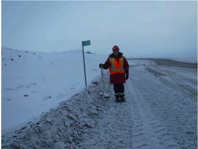
Photo 5-5 Snow bank heights measured from the road surface up to the top of the bank on both the east and west banks at set locations (km 06), November 3, 2018.
