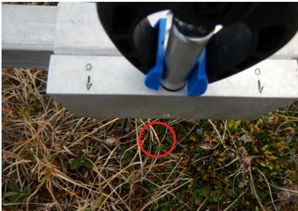
Photo 4-4 A view showing the diameter of the laser projecting onto the vegetation (2 mm), 27 July 2014.
