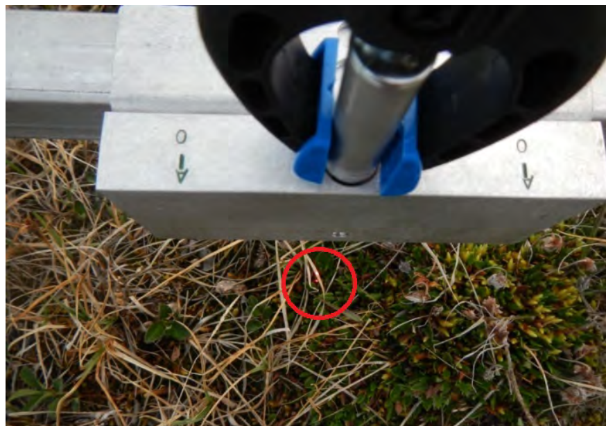
Photo 4. A view showing the diameter of the laser projecting onto the vegetation (2 mm), 27 July 2014.
