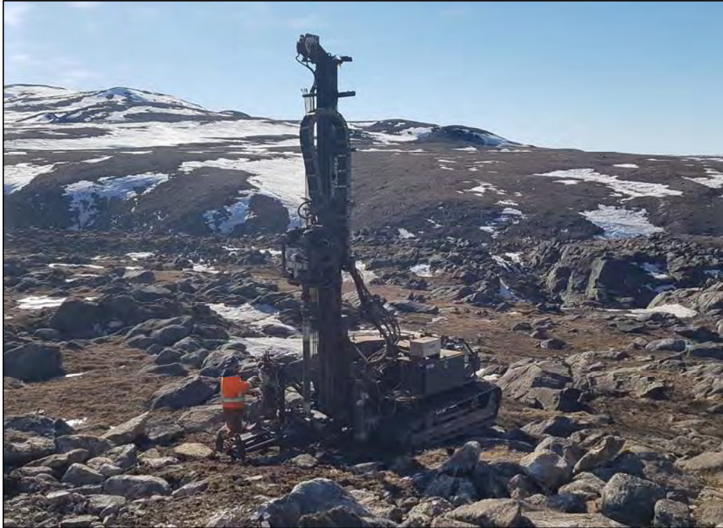
PHOTO 3 - KM106-DH19-01 Looking South During Drilling
