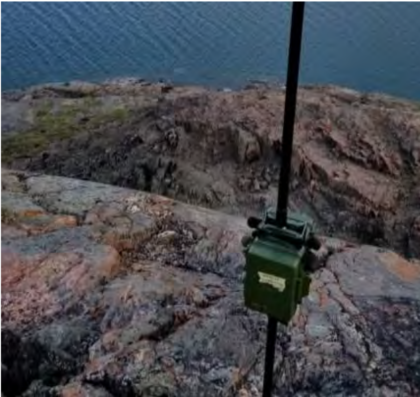
Photograph 4.3: Two SM4 acoustic recorders mounted back-to-back on a fiberglass pole. The shoreline location of the Inuit hunting camp is visible in the background.
