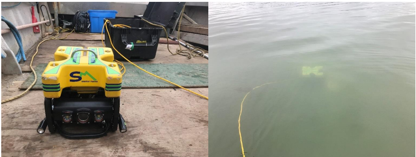
Figure 1: Seamor Chinook 300F ROV on deck of vessel (left) and during ROV survey (right)
