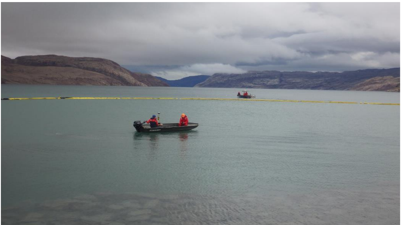
Photo 56 - Allnorth surveyors performing bathymetry survey of dredge area, 11 July 2019
