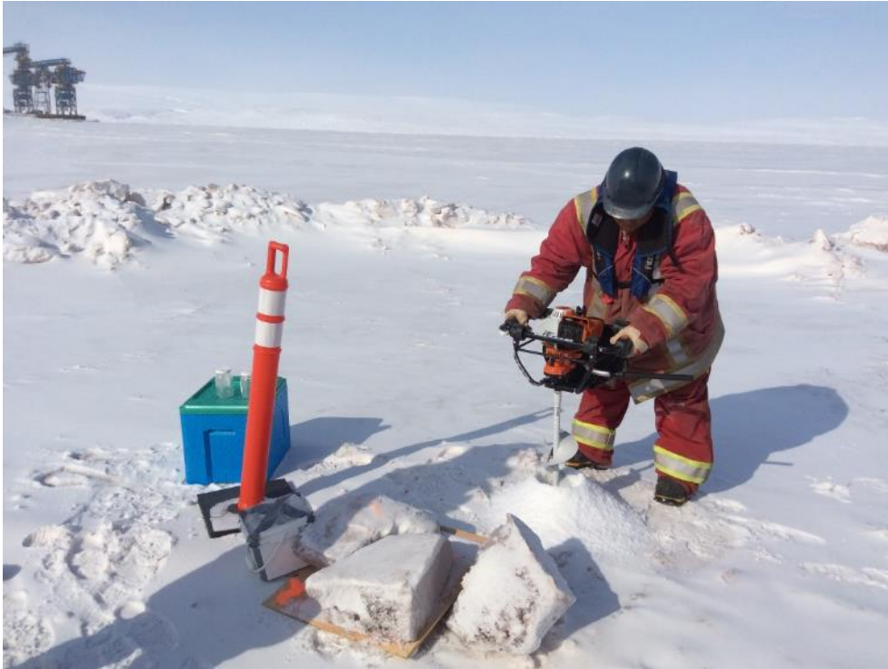
Photo 13 - Augering of a hole through sea ice at a turbidity monitoring location, 25 April 2019
