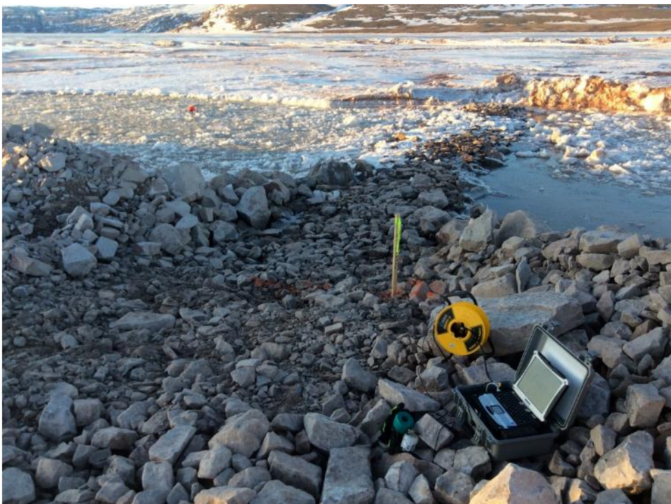
Photo 24 - Underwater noise monitoring conducted during ice breaking and removal activities with an excavator. Hydrophone deployed from red buoy within cleared ice area, 13 May 2019
