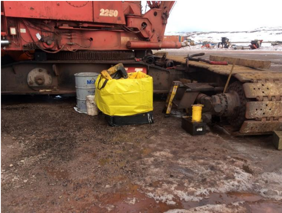
Photo 21 - Spill containment material on hand during engine removal work on the 2250 Manitowoc crane, 9 May 2019
