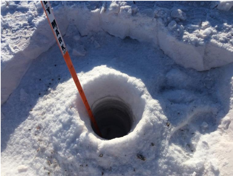
Photo 9 - Ice profiling hole showing 0.7 m of ice thickness. The minimum ice thickness required for the necessary equipment load is 0.55 m, 13 April 2019
