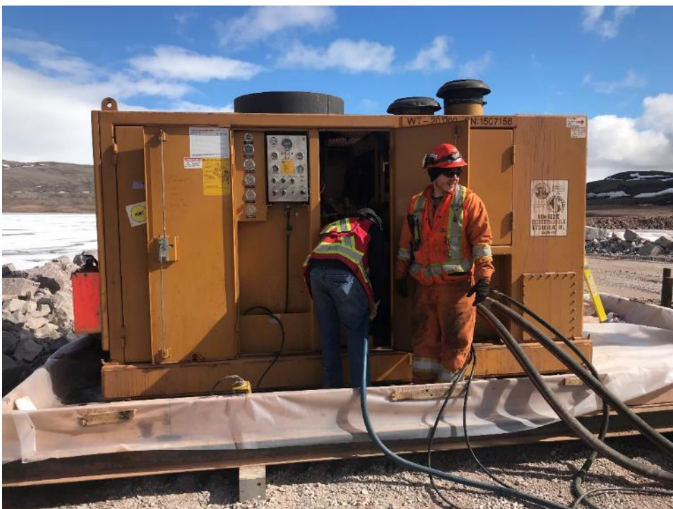
Photo 36 - Fueling of the vibratory hammer hydraulic power pack, 5 June 2019
