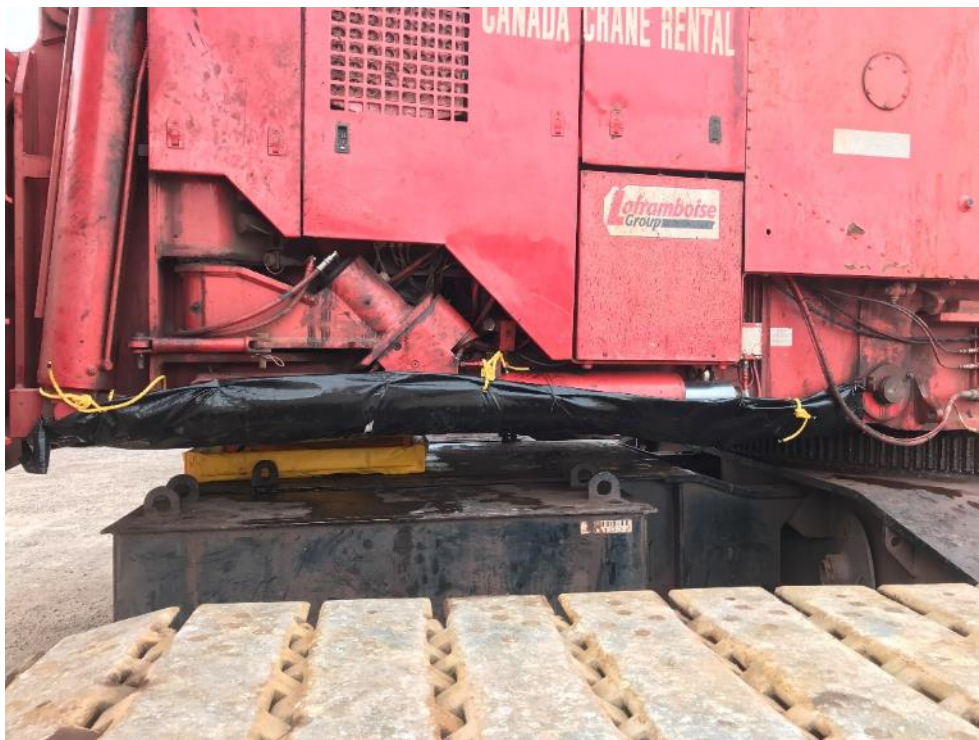
Photo 32 - Full time spill containment (black tarp and yellow rope) attached to underside of 2250 crane, 31 May 2019
